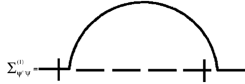
FIG. 2. The one-loop self-energy graph for \Sigma_{\psi'\psi} . The lines correspond to propagators (6) and (8). Slashes denote the end carrying arguments of the field \psi' ; plain end carries the arguments of the field \psi . Vertices correspond to the factor V_{ijs}=ik_j .
